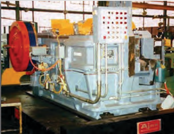
Typical 2" Ajax Forging Machine
