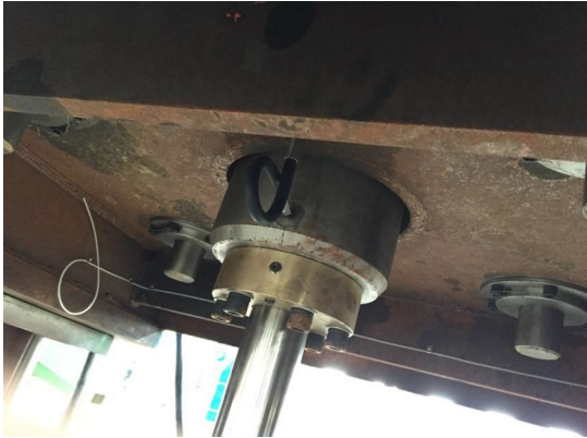
Ajax-CECO flexible hydraulic cylinder is not directly welded to the top limit block, allowing it to flex.
