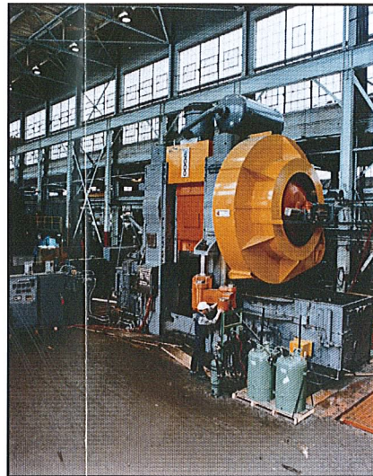
6,000 ton Automated Forging Press System
