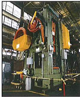
4,000 ton Ajax retrofitted with hydraulic wedges and knockouts, controls and updated lube system.
