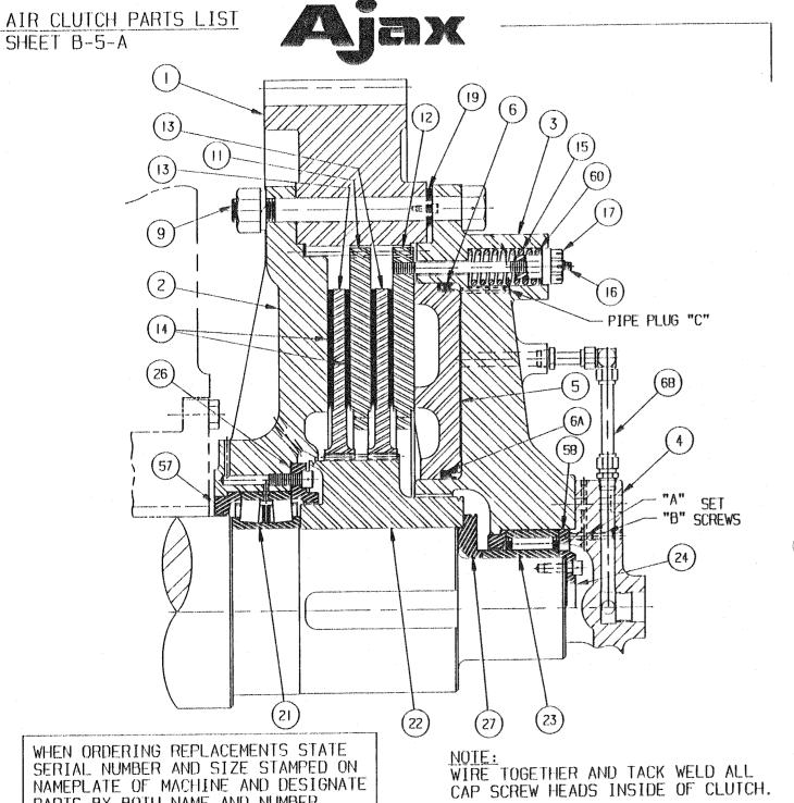
SERIAL NUMBER AND SIZE STAMPED ON NAMEPLATE OF MACHINE AND DESIGNATE PARTS BY BOTH NAME AND NUMBER
