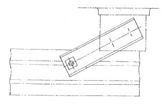
AFTER BRAKE SUPPORT IS ASSEMBLED, ADJUST "A" FOR 16" GAP BETWEEN WASHER (1296) AND BRACKET (1295) WITH BRAKE SET. ADJUST "B" TO TIGHTEN SPRING (1294) JUST SUFFICIENT TO BRING WASHER (1296) AGAINST BRACKET (1295) WHEN BRAKE IS RELEASED.
